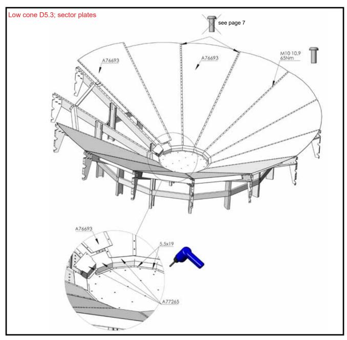
Install the sector plates on top of the sector beams. Do not yet install the uppermost and the lowermost bolts for the sector plates at this stage. Use cup-heades screws for fixing the sector plates. Do not tighten the bolts until all the legs and the sector plates are in place. Before completing the assembly of the cone, lift the remaining parts inside, and install the last wall panel for the silo.
