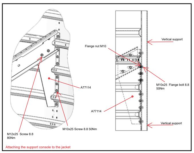
Install the support console A77114 in the same position with the vertical support for the silo jacket. Determine the correct installation height of the console by checking the distance between the rolls in the drawings. (See page 7). Attach the support console to the silo jacket using M10x25 flange bolts: 8 pcs/bracket. Join the support console, silo jacket and the vertical support together using bolts.
