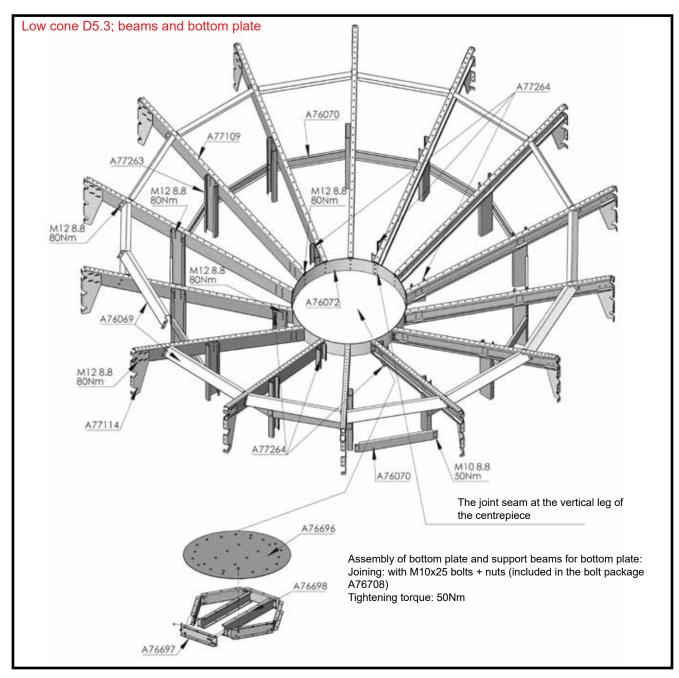
There are in total 6 inner legs A77264, so each horizontal beam will not be provided with an inner leg. The mutual distance of the inner legs A77264 shall be as illustrated in the drawing. The joining seam of the centrepiece (A76072) must be positioned at one of the vertical legs.
