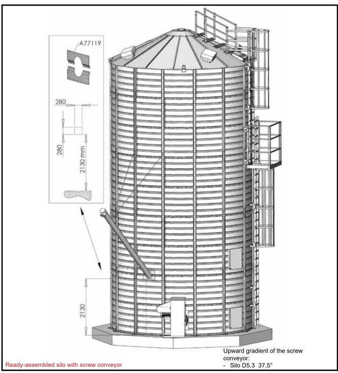
Make a hole in the jacket plate of the silo for the emptying screw, see drawing. Observe the positions of the support legs for the cone. Seal the lead-through using the cover plates A77119. Support the screw conveyor, for example, by means of wire ropes, as illustrated in the drawing.
