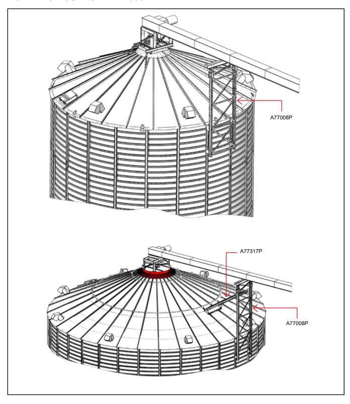
Diagonal A77317P is not included in the conveyor support A77008P structure. (If required, order separately.)
