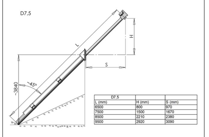
Installation height of the wall joint for the screw conveyor
