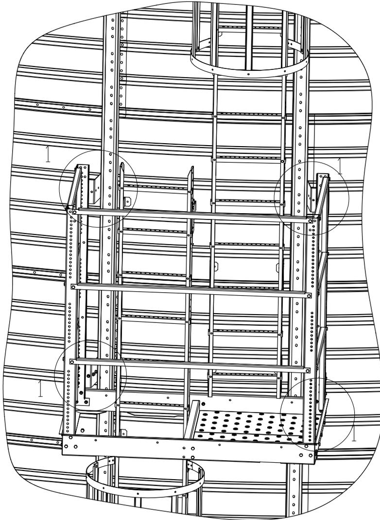
The landing is mounted on the vertical supports. Attach the platform to the vertical supports using fasteners (A76322 4pcs.) in all.
