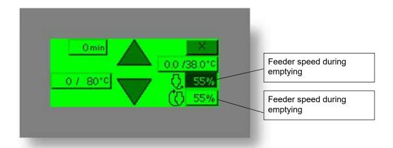
If grain level reach silo top sensor, screen below show up. When selected silo is full, emptying function can be quit or divider position can be changed to other silo and continue emptying.
