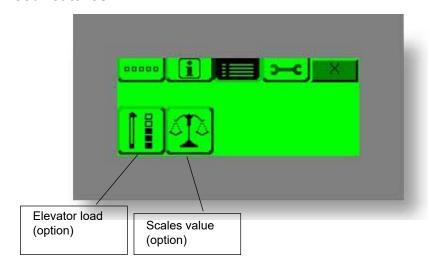
Elevator load meter shows elevator load as current and percentage of full load (option).
