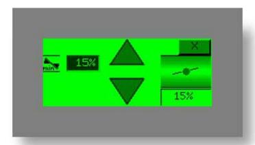
Setting of automatic filling (option) defines starting point of drying. If program with filling and drying functions is selected on functions screen, on settings it is possible to select start of drying when grain level reaches middle level sensor of top level sensor.
